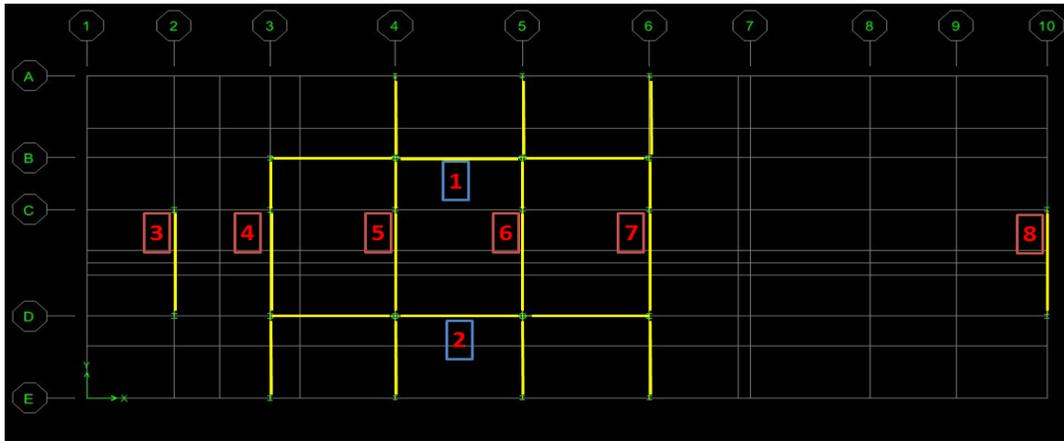
Figure 17: Lateral Frame Layout & Notation
