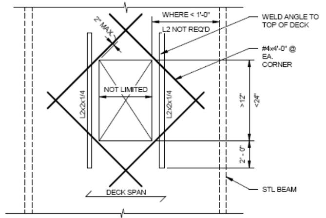
Figure 4: Openings in Slab on Steel Deck
